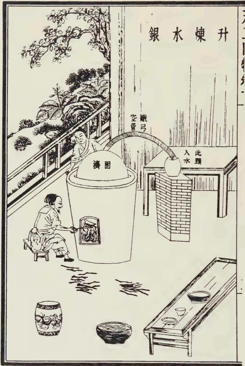
Fig. 92. Retort still for mercury, from the Thien Kung Khai Wu of +1637 (Chhing drawing).
